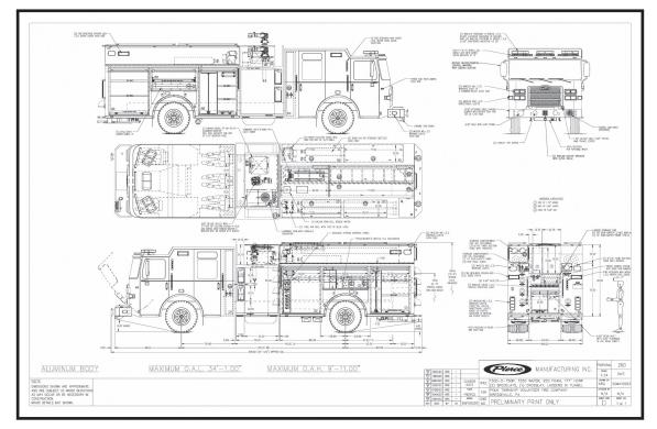
Above is the approved design for our new 2027 Pierce Enforcer Heavy Duty Rescue Pumper, it has a 750-gallon water tank, 1500 GPM Hale Pump, 25-gallon foam tank, seating for 5 firefighters, equipped with both firefighting equipment, vehicle stabilization and rescue equipment as well as a cascade system for clean breathing air.
